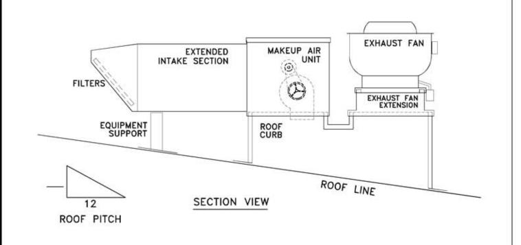
ROOFTOP FAN PACKAGE COMBINATION ROOF CURB MODEL RCC
